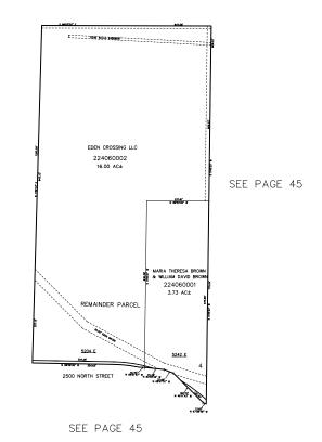
10' UTILITY & DRAINAGE EASEMENTS EACH SIDE OF PROPERTY LINES AS INDICATED BY DASHED LINES EXCEPT AS OTHERWISE SHOWN.
